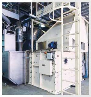
Drying and cooling: Dryer for kibbles.
