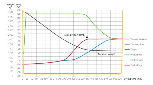
Typical drying times for raw meat products range from 8–16 hours depending on the allowable product temperature and the water content. Most pet food product can be dried in less than 12 hours. During drying the temperature is constantly monitored and the system automatically regulates to avoid scorching the product.
