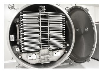
The overhead rail system for loading and unloading, and the Continuous De-Icing system, enable a changeover time between batches of under 30 minutes.
