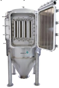
Less complicated than competitive products, the hinged tubesheet provides a single point of access to the baghouse section through the clean air plenum; eliminating additional platform or mezzanine access requirements.
